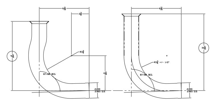
1928 Inlet Pipe on left, April 1929 to end of production on right.
